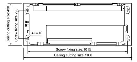
Please accord to the follow figure's requirements to design the length of the suspender bolt.
