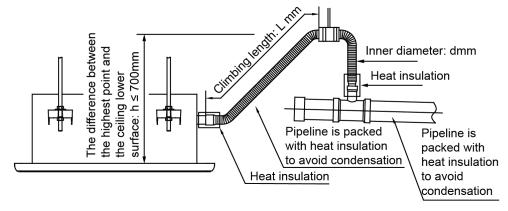
Please according to the tube hardness to choose proper support density, do not appear obvious dropping and deformation situation. Dropping part will save the water and lead to poor drainage and abnormal noise.
