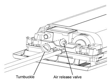
• When finished pipes and junctions connection. Turn the turnbuckle down, find the air release valve inside the unit, and exhaust the air contained in the circuit.
